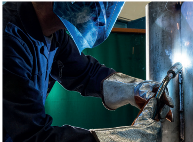
MAG welding of stainless steel
